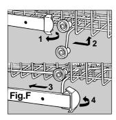
Open the rail stop flaps and pull the basket out completely. Now place it in high or low position, then slide it along the guide rails until the front wheels also go in. Now close the rail stop flaps. Follow the sequence of actions illustrated in figure "F".
